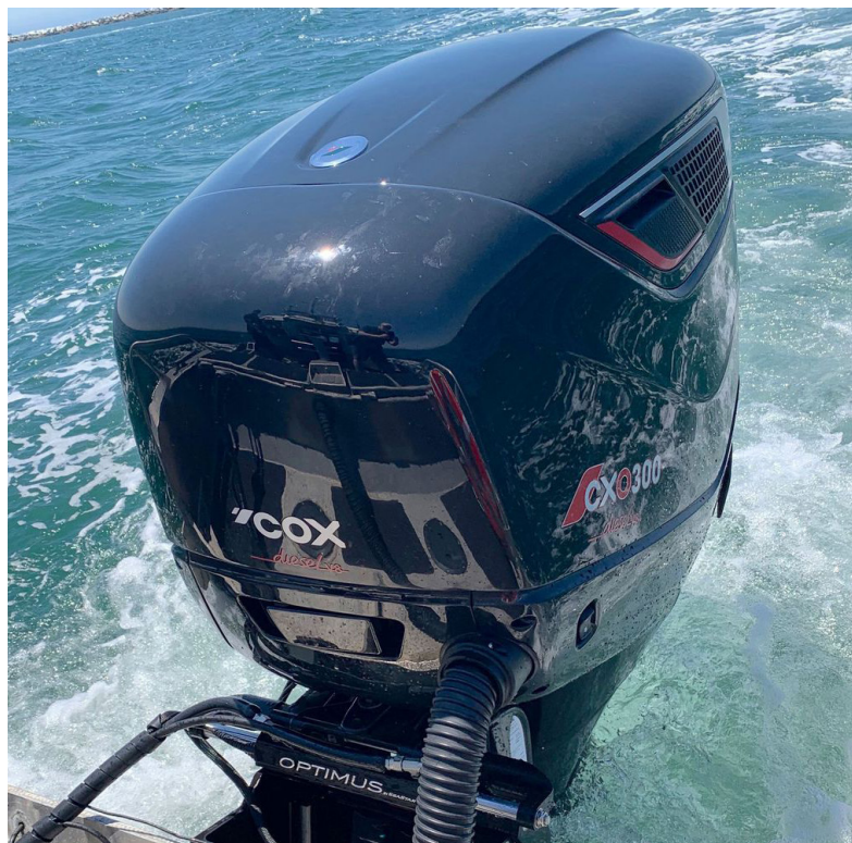
The single CXO300 powered the Safe Boat S25 to speeds over 40 mph at wide-open throttle and achieved optimum fuel efficiency of 3.3 mpg at 29.7 mph. - Jim Hendricks / Sport Fishing.
