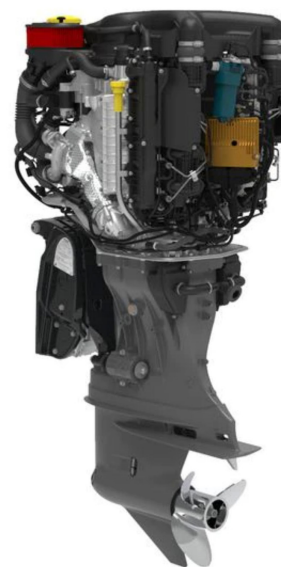
The Cox diesel outboard uses twin turbochargers to deliver a pressurized charge to each cylinder bank of the V-8 diesel powerhead. - Courtesy Cox Powertrain.
