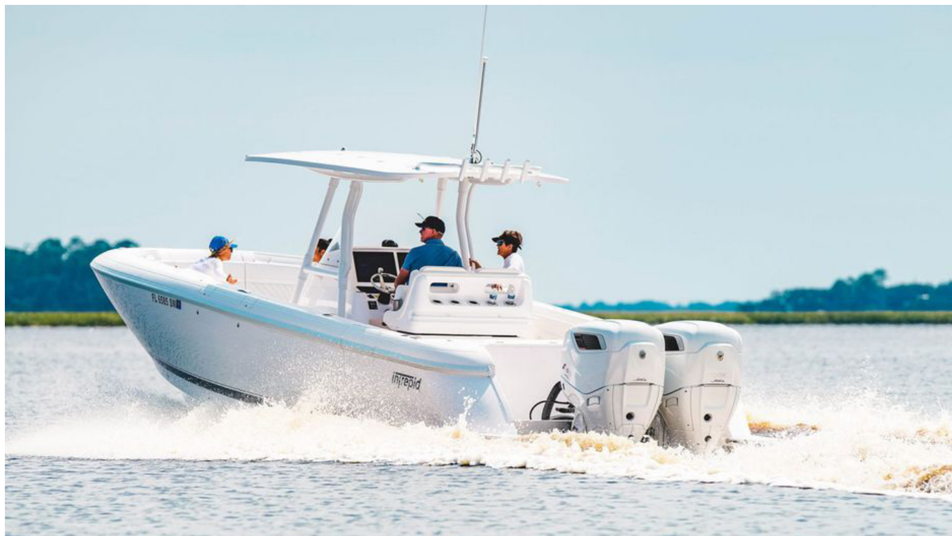
Cox Powertrain has worked closely with Florida-based Intrepid Powerboats in developing and refining the CXO300 diesel outboards for center-console fishing boats such as the 345 Nomad. - Courtesy Cox Powertrain.
